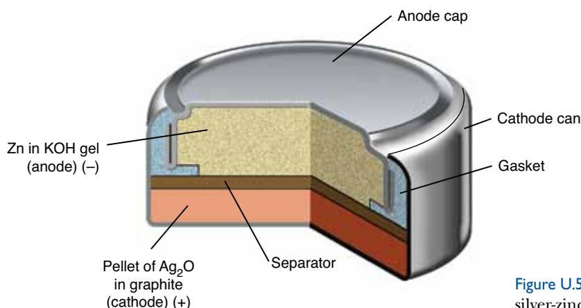
Figure U.5 A cutaway view of a typical silver-zinc button battery.
