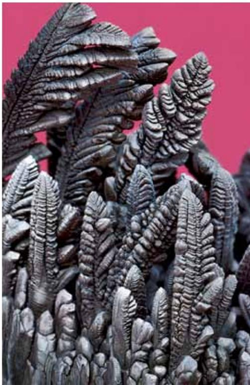
**Figure U.2** Metallic dendrites formed during electrochemical deposition. Such dendrites occur in the rapid discharge of a lead storage battery and can lead to an internal short circuit.
